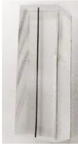
Figure 3-10 (a) Schematic and (b) photograph of compression specimen for a single FDM filament.
