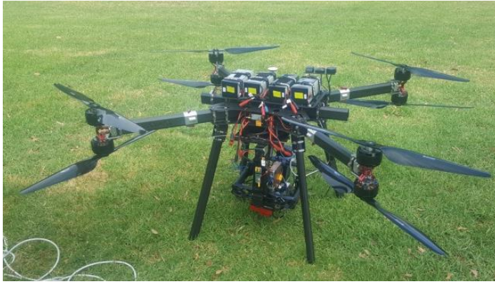
Figure 4.5. Drone with LiDAR sensor used to capture points cloud from plan view.
