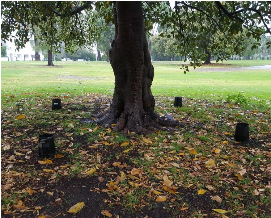
Figure 4.3. Arrangement of tipping buckets.
