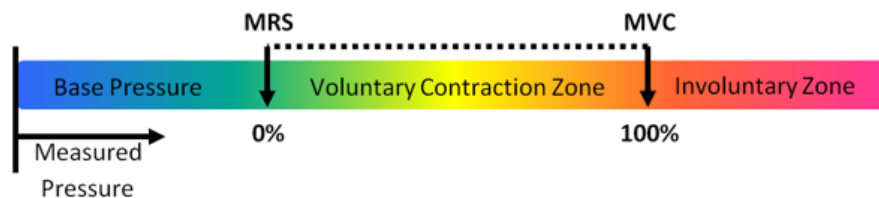
Figure 3.7: Measuring MVIC through garment pressure range
