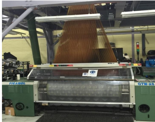
Figure 9.27: Jacquard weaving machine (Picanol GTM – AS)
