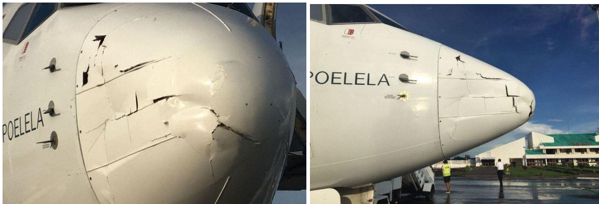
Fig. 1.1: Impact damage to the composite nose dome to a Boeing 737-700 aircraft [5].
