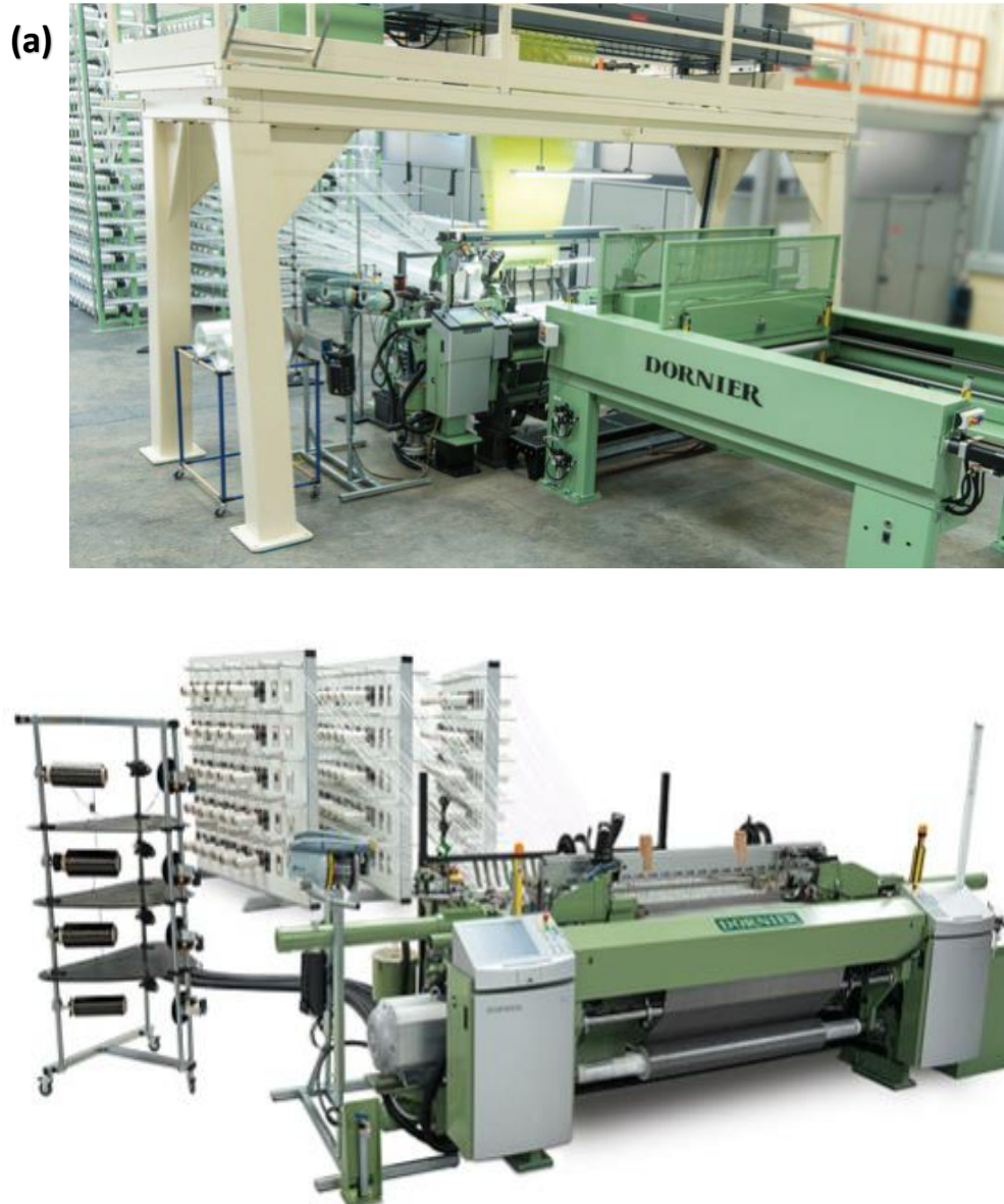
Fig. 2.2: 3D weaving looms for 3D woven fabric manufacturing based on (a) Jacquard and (b) rapier principles [22].
