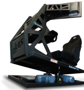
FIGURE 2 “Thruxim” 2DOF motion simulator
